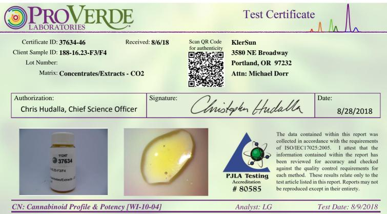
The client sample was analyzed for plant-based cannabinoids by Convergence Chromatography (CC). The collected data was compared to data collected for certified reference standards at known concentrations. Estimation of exo-THC signal is 0.5%, based on area relative to THC standard.
